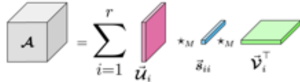
Figure 5: Expansion of t-rank-1 tensors derived from slices of \mathcal{U} and \mathcal{V} with diagonal tubes of \mathcal{S}
