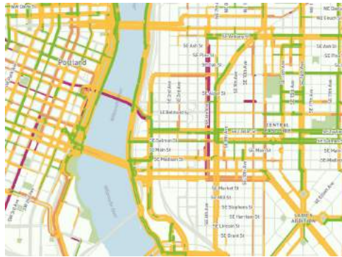
Figure 1: Ride Report's Stress Map for Portland, OR. Greener road segments indicate less stressful streets while more red segments indicate more stressful streets. "Stress" is computed by taking the average rating for each segment.
